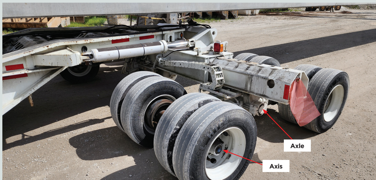
Figure 10. Definitions of axis and axle in Trail King TK170SD trailer.
