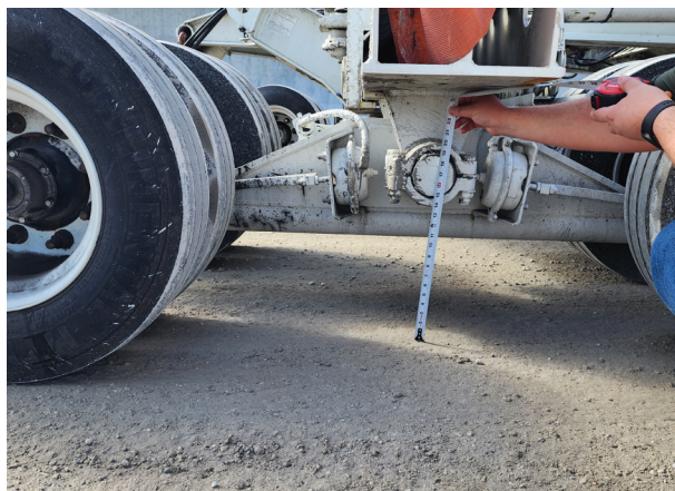
Measurement at the jeep or dolly leaf suspension
