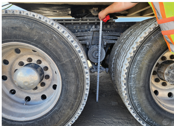
Measurement at the truck leaf suspension
