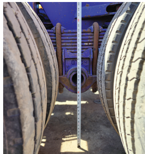
Height measurement at the leaf suspension
