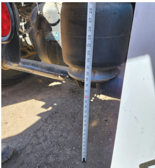
Height measurement at the air suspension
